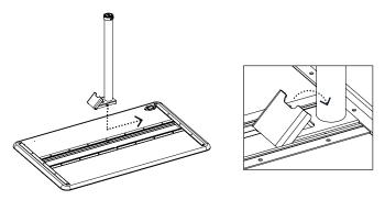
Align the knobs inside the foot with the notches on the leg cap. Rotate the foot 90° until you hear the click of the release button. (To remove the foot, press the release button.)
