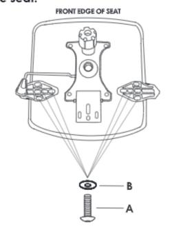
2. Screw in 3 bolts to secure the back to the seat.
