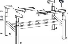
11. Slide the brackets onto each leg structure and attach each with 2 screws.
