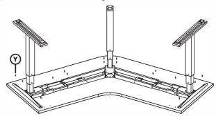
10. Shift the spanning rail position as necessary to center the arrows between the leg frames.
