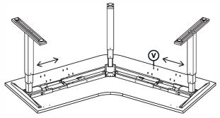
11. Slot the control box into G3 leg frame. Attach control handset with two screws, using the pre-drilled holes.
