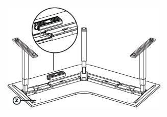
12. Complete the cable connections between the control box, legs, and handset.
